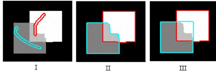
**Figure 14.** Solutions computed using (4.1) and (6.1) for spectral noise images. (I) Image of 2 objects (white and dark gray) with noise induced edges (due to the light gray region). (II) Incorrect result using (4.1) (segmentation of cyan curve influenced by image term). (III) Correct result using (4.1) (segmentation of cyan curve influenced only by shape term).
