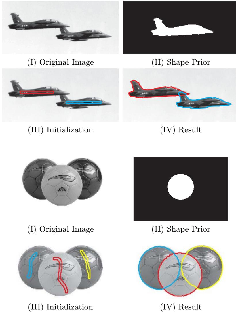
**Figure 10.** Segmentation results for real images of multiple objects under occlusion. (I) Input image to segment. (II) Explicit shape prior to be used for segmentation. (III) Initial contours that have to be placed close to the objects. (IV) Correct result with use of a shape prior.
