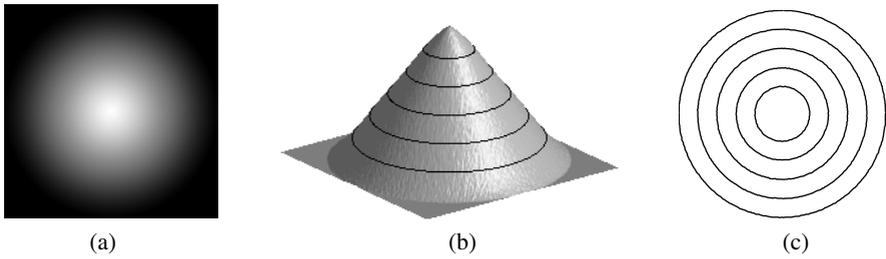
**Fig. 1.** (a) A synthetic image of a circular object with a gradual intensity fall from the centre toward the boundary. (b) The image surface of (a) in a three-dimensional space and heights to be quantised are marked on the surface. (c) Contour map generated from quantisation in (b).
